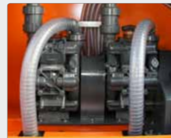
Logically built liquid system featuring diaphragm pump.
