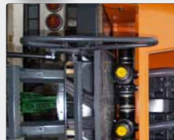
Service-friendly machine house permitting quick access to computer unit, valves and liquid pumps.
